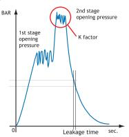
from that moment the test cycle automatically alternates the chatters at the first and second pressure stage. DIT31 display these values with the parameters P1 and P2. For each chatter, DIT31 also calculates the K factor as a reference of the flow.
