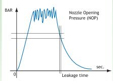
The cycle stops by pressing the STOP command. DIT31 calculates the leakage time as evidence of the nozzle seat leakage.
